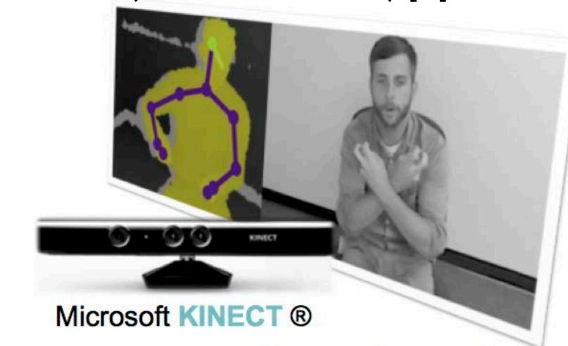
ChronoSense tool captures the RGB image recorded from Kinect.
